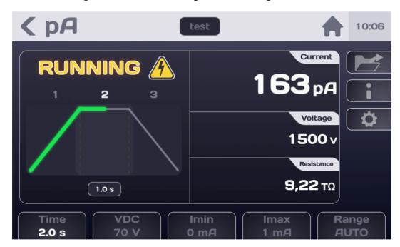
At the end of the test the display indicates if the measurement is between Imin and Imax, i.e. considered as PASS.
