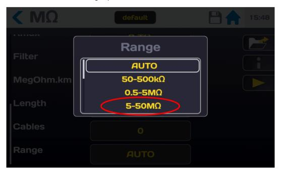
Select the resistance range, the max. value indicated is equal to: Voltage / Imin and the min. value is equal to Voltage / Imax. With the following current ranges:
