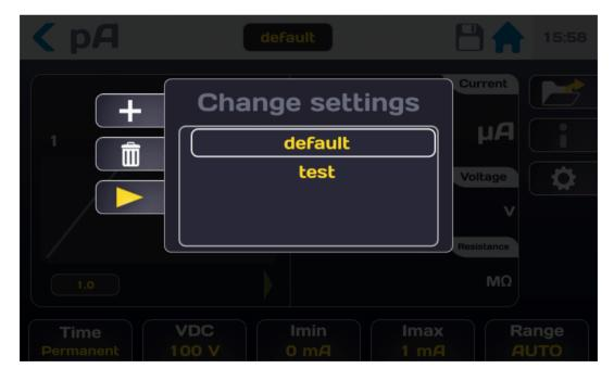
Search for the filename by scrolling up or down in the list of files. Press the desired filename then press outside of the file list display area or on the button with the yellow Arrow.
