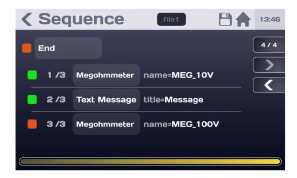
In this example, the result of the sequence is BAD because of step 3/3 measurement in Megohmmeter mode with the parameter file "MEG\_100V".
