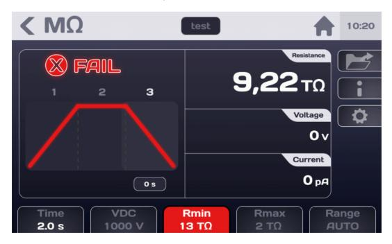
The coloured parameter shortcut button will indicate the parameter which causes the FAIL result for the measurement.
