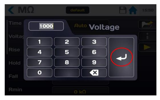
Enter a voltage value between 1 and 1,500 VDC, if the value entered is outside of the authorised limits it will turn red. Press the Arrow validation button to confirm the new value and return to the previous menu.
