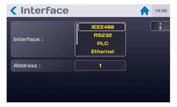
SEFELEC1500M test and measuring instruments can be equipped with an interface of the IEEE488 type. It allows all of the instruments in the range to be integrated into an automatic test or measuring system, whether intended for manufacturing control or for input control. The interface can be accessed through a connector located on the rear panel of the device.
