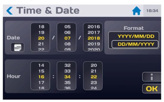
Select the date format YYYY/MM/DD or DD/MM/YYYY then set the date using the drop-down windows or press the icon symbolising a calendar to select a date directly.
