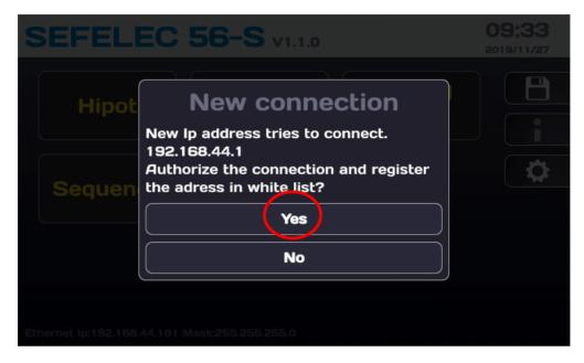
If the IP address is a known address, then validate the connection request by pressing YES to add the IP address into the list of permitted addresses (white list), if not press NO. Then repeat a connection attempt which will be accepted by the device without repeating the
