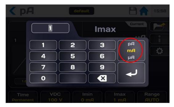
Enter the threshold value by using the Pico, Nano, Micro, Milli ampere units.
