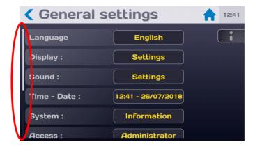
To scroll the screen down, place your finger towards the bottom of the screen and while remaining in contact with the screen, swipe towards the top of the screen with your finger; swipe in the opposite direction to scroll the screen up.
