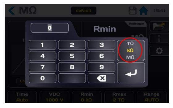
Enter the threshold value by using the Tera, Mega, Giga or kilo  $\Omega$  units.
