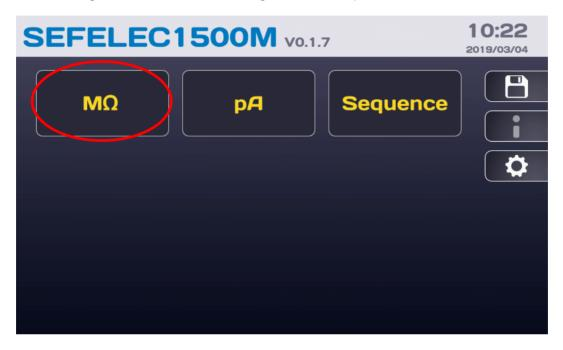
press the  $\mathbf{M}\mathbf{\Omega}$  button to access the following measurement screen:
