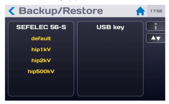
Choose the file by pressing on its name and drag it from the Device column to the USB Key column or vice versa depending on the desired operation. A message confirming if the copy operation has been successful is displayed briefly.
