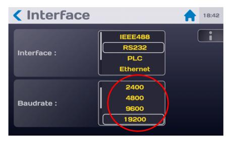
A command destined for the device must end with the character: LF (hexadecimal 0A, decimal 10). The codes can be sent in upper case or lower case. The maximum number of commands in the same block must not exceed 15 instructions. Take care not to associate normalized orders or queries with other types of commands.
