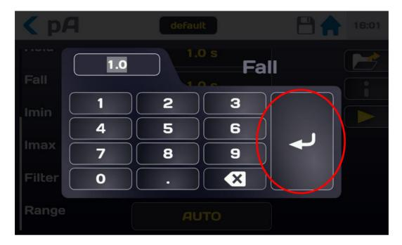
Enter the value of the time in seconds: if the value entered is outside of the minimum and maximum limits it will be displayed in red. Press the Arrow validation button to confirm the entry and return to the configuration menu.
