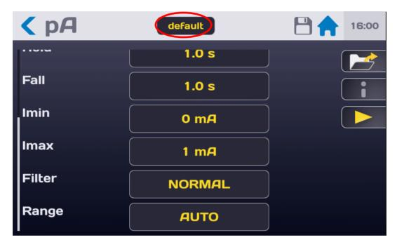
To change the filename, press the area with the filename in order to display a virtual keyboard and enter the new name.
