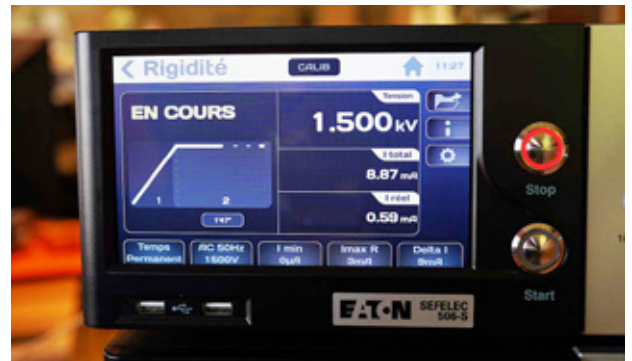
SEFELEC 506-S performing hipot test displays real and total currents
